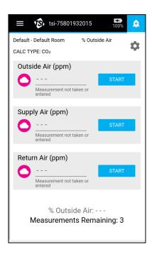
As mentioned above, three measurements are necessary for % **Outside Air** calculations - **Outside Air**, **Supply Air**, and **Return Air**. The measurements may be taken in any order. The calculation is performed once the final measurement is taken.
