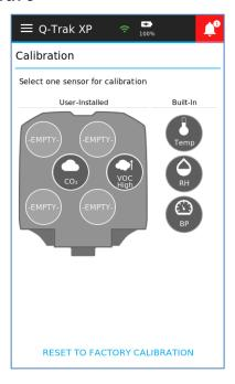
Step 1 – Select a Gas Sensor for Calibration
