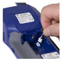
Insert the battery as shown in the picture, keeping the battery wires to the side and clear of the battery cover screw.
