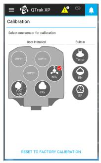
An Out-of-Range error during the calibration of a sensor means the sensor's offset or calibration slope adjustment has drifted outside of the TSI® recommended specification for continued use. Sensor should be replaced or sent to TSI® for re-calibration.
