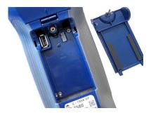
2. Connect the battery to the handle connector.
