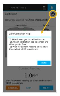
necessary. See Table 1 for recommended ZERO and SPAN gases.
