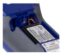
Attach the battery compartment cover, ensuring battery wires are clear of the screw.
